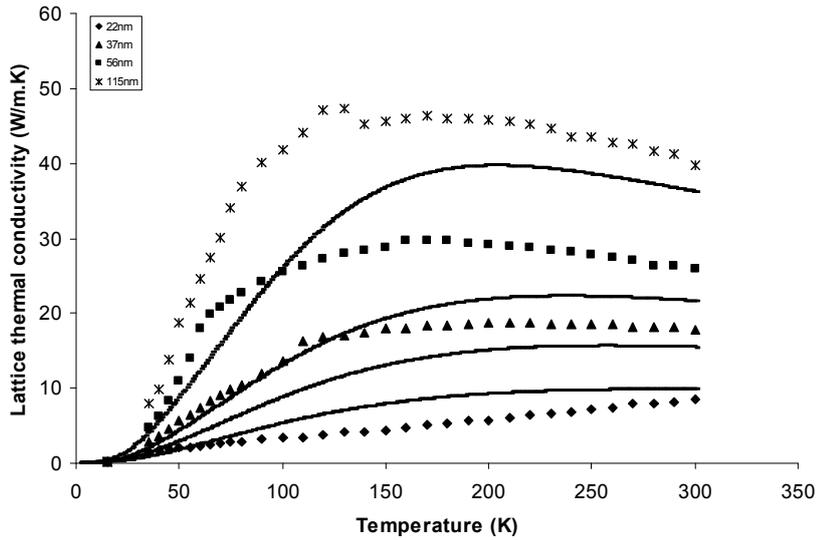
**Fig. 1.** Calculated lattice thermal conductivity versus temperature from 2 to 300 K for silicon nanowires of diameters 22, 37, 56 and 115 nm by using the effect of all scattering and calculated phonon group velocity, Debye temperature and melting point in comparison with that of the experimental data[11].
