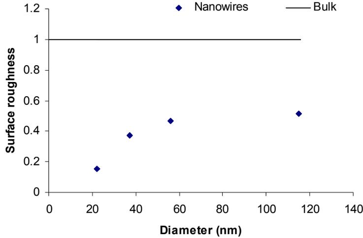
**Fig. 4.** The surface roughness versus silicon nanowire diameter.
