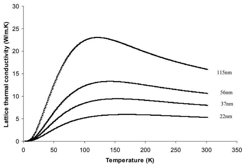
**Fig.2.** Calculated lattice thermal conductivity versus temperature from 2 to 300 K for germanium nanowires of diameters 22, 37, 56 and 115nm by using the effect of all scattering and calculated phonon group velocity, Debye temperature and melting point.
