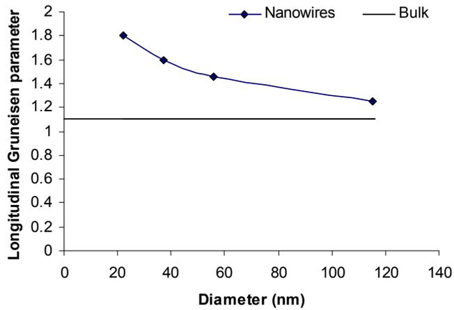
*Fig.5. The longitudinal Gruneisen parameter as a function of nanowire diameter for silicon.*
