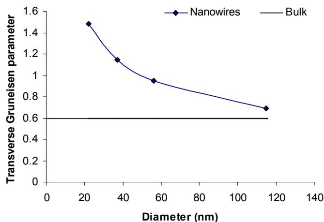
*Fig.6. The Transverse Gruneisen parameter as a function of nanowire diameter for silicon.*
