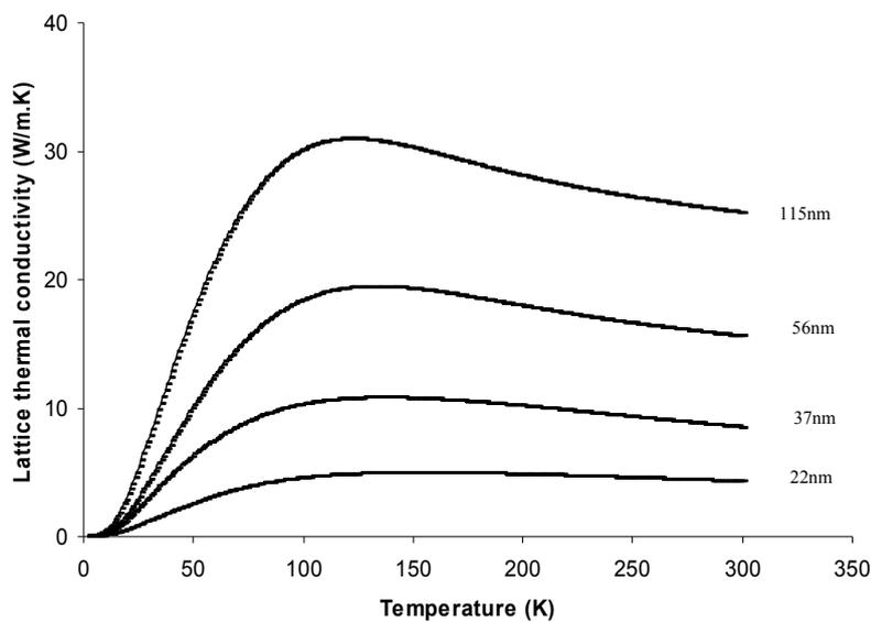
**Fig.8.** Modification and recalculation lattice thermal conductivity versus temperature from 2 to 300 K for germanium nanowires of diameters 22, 37, 56 and 115nm by using the effect of all scattering and calculated phonon group velocity, Debye temperature and melting point well as the size dependent parameters of lattice dislocation, surface roughness and Gruneisen parameter.
