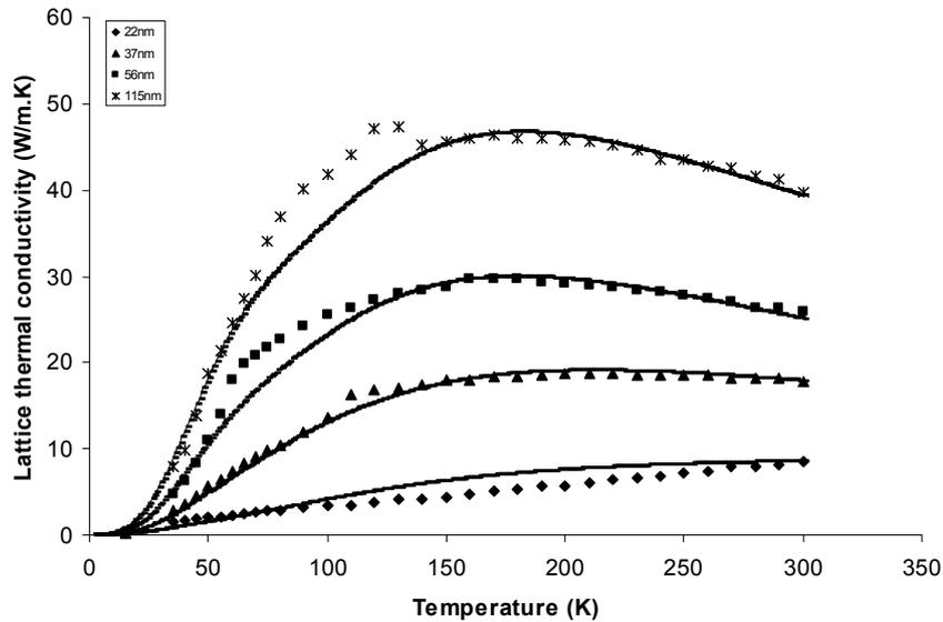
**Fig.7.** Calculated lattice thermal conductivity versus temperature from 2 to 300 K for silicon nanowires of diameters 22, 37, 56 and 115nm by using the effect of all scattering and calculated phonon group velocity, Debye temperature and melting point as well as the size dependent parameters of lattice dislocation, surface roughness and Gruneisen parameter in comparison with that of the experimental data [11].
