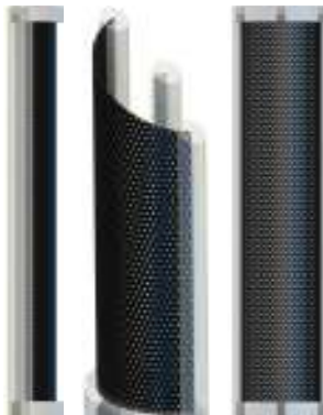
Fig. 1. Ionic loudspeaker of cylindrical geometry (side and front views).
