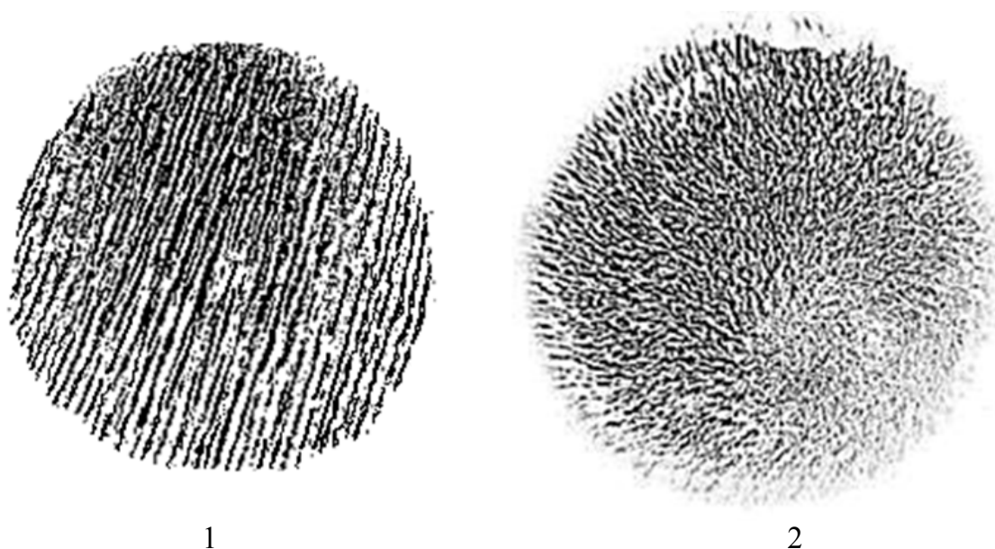
Fig.1. Radiographs of sample PCM disks with "fibers" oriented: 1) in the disk plane and 2) normal to disk.
