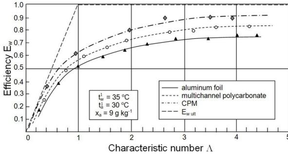
Fig. 4. Efficiency of the water cooling process in CTW.
