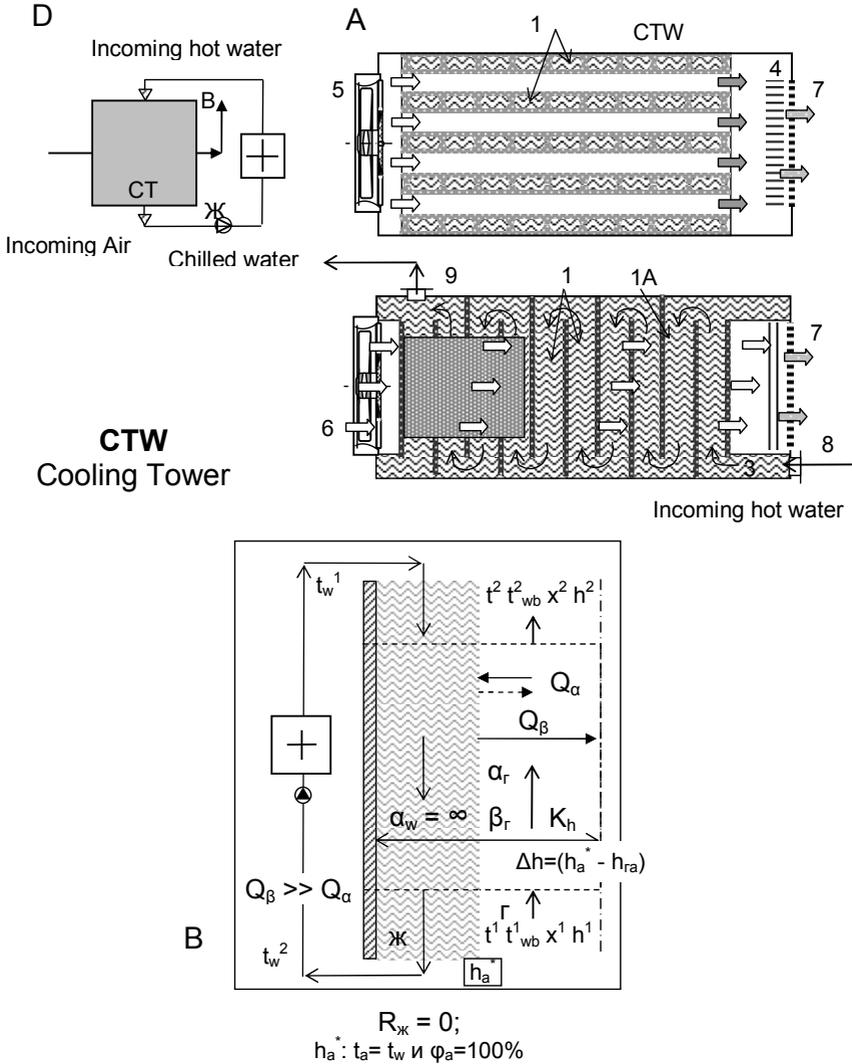
**Fig. 6.** Direct evaporative cooler of water DECw (Cooling Tower, CTW) on the basis of plate ceramic microporous multichannel structures. Designations are according to Fig. 7. Additional: 7 – exhaust air; 8 – incoming hot water from sunliier; 9 – chilled water
