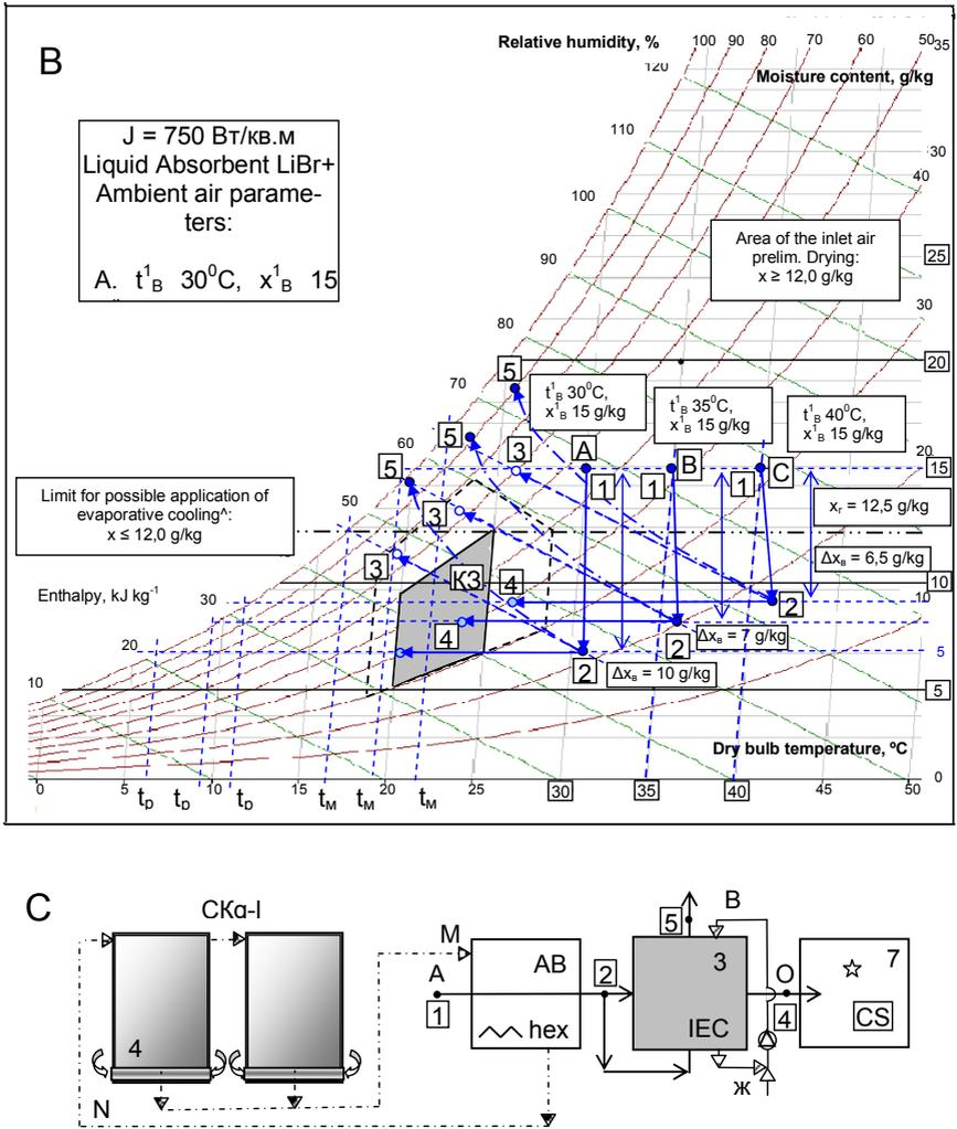
**Fig. 9.** Perspectives of the solar cooling system intended for air conditioning on the basis of open absorption cycle with direct solar regeneration of the desiccant (B) for the formulae of the system ABR-IECg. Solar cooling and air conditioning systems (Solar-EC)
