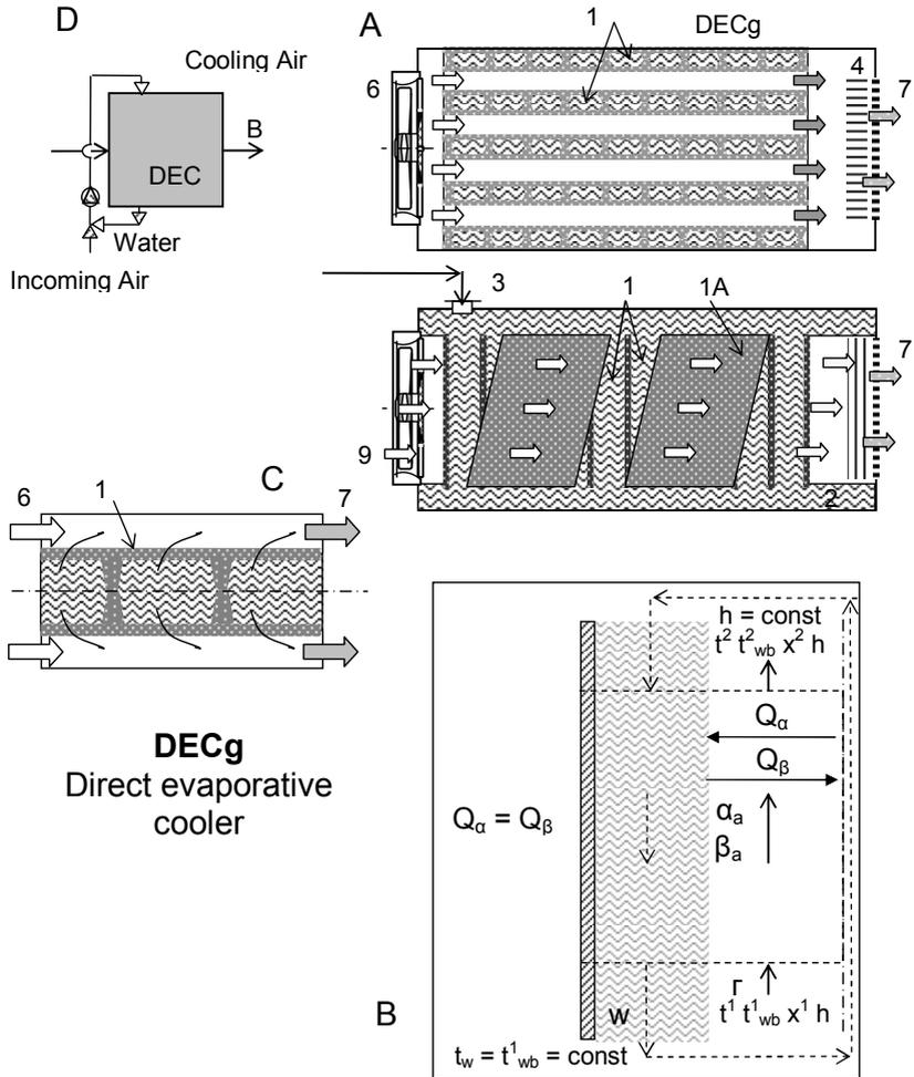
**Fig. 5.** Direct evaporative cooler of air DECg on the basis of plate ceramic micro-porous multichannel structures.
