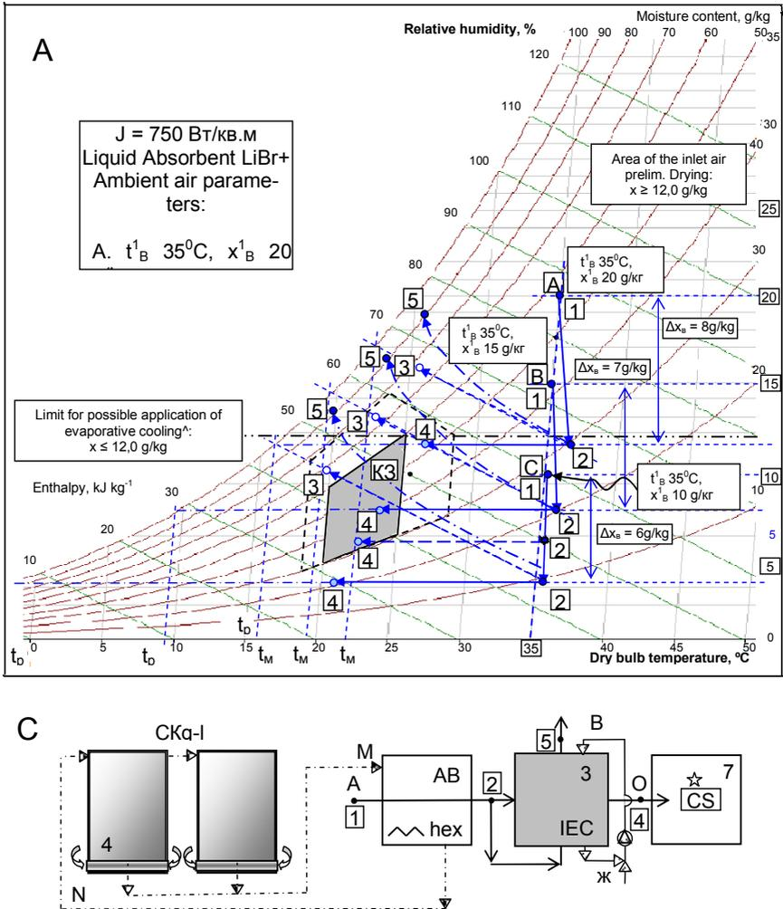
**Fig. 8.** Perspectives of the solar cooling system intended for air conditioning on the basis of open absorption cycle with direct solar regeneration of the desiccant (A) for the formulae of the system ABR-IECg. Solar cooling and air conditioning systems (Solar-EC)
